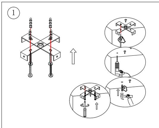
Take out the cross hanging board, and fix the cross hanging board at the position where the ceiling appears.
