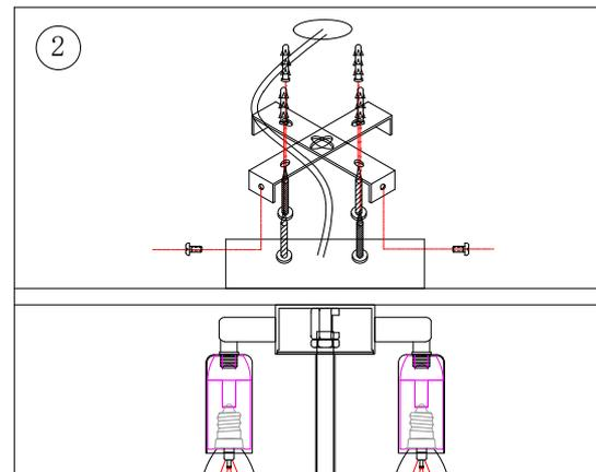
Connect the power cord, fix the ceiling plate on the hanging board with screws on the side / install the light source and try to light it
